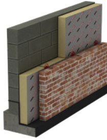
Partial Fill Cavity Wall
