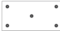
5 No. per board (1.2 x 0.6 m board - 6.94 fixings / m 2 ) (1.2 x 1.2 m board - 3.47 fixings / m 2 )
