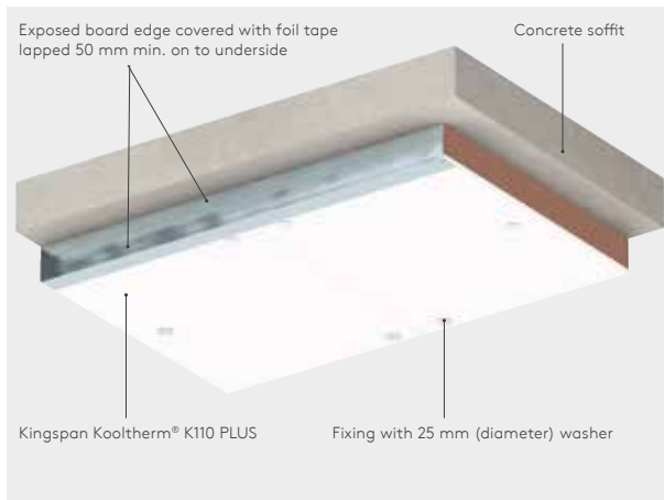
Figure 2: Protection of exposed insulation edges of Kingspan Kooltherm® K110 PLUS
